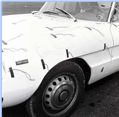
Prototype undergoing wind testing at the Balocco test track in 1965
