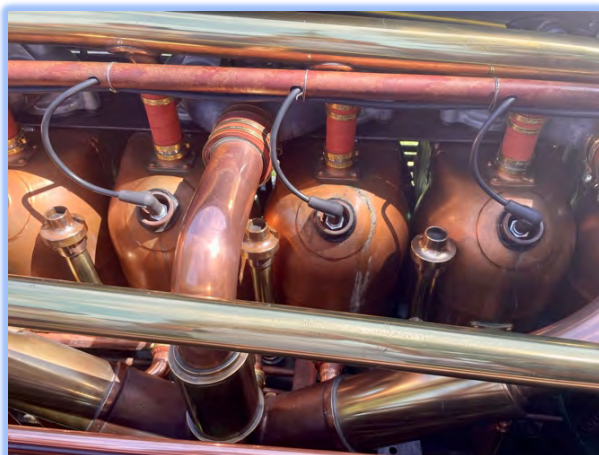
Extensive use of copper tubing, both as an engine housing design feature and to provide an effective radiator, is one of the many remarkable period characteristics to be seen on Peter Briggs’ very dramatic 1904 Napier.
