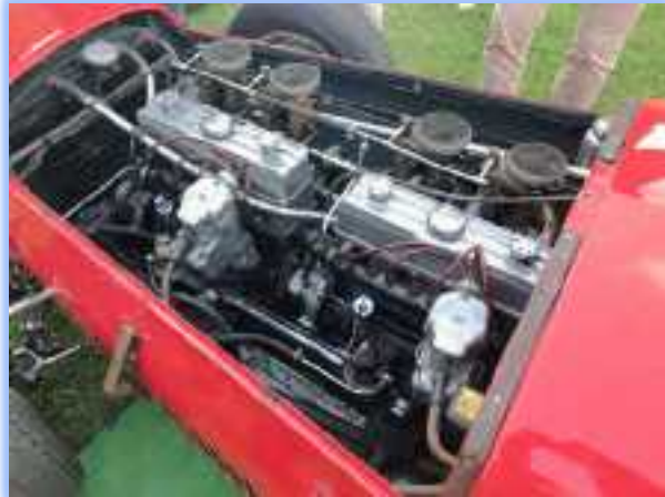
The remarkable 8C Bi-Motore engine with its separate Fiat 1100cc engines and special coupling.
